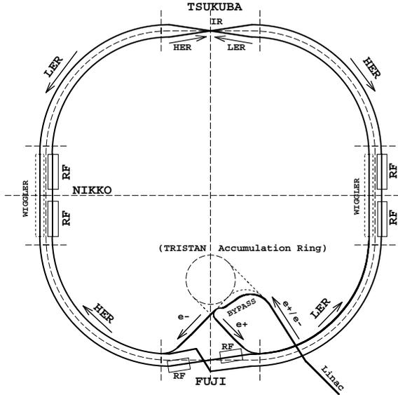
Figure 1.2: Configuration of the KEKB accelerator system
