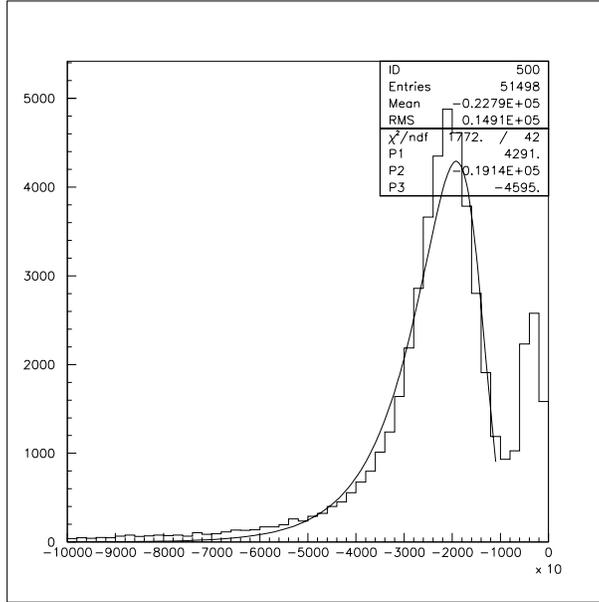
Figure 4.7: Pulse height distribution for p-side
