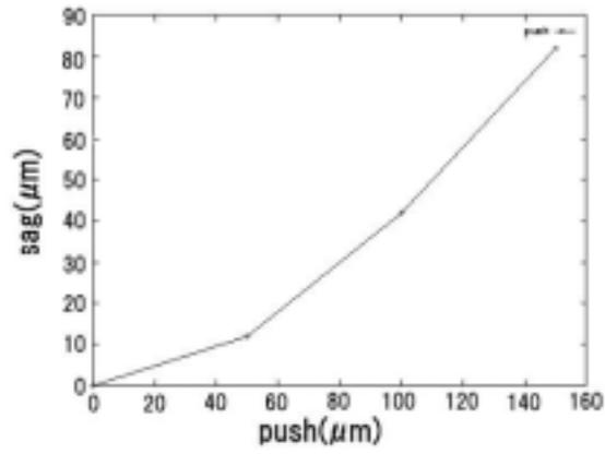
Figure 3.26: The sag of the center of the ladder when we push the ladder from one side
