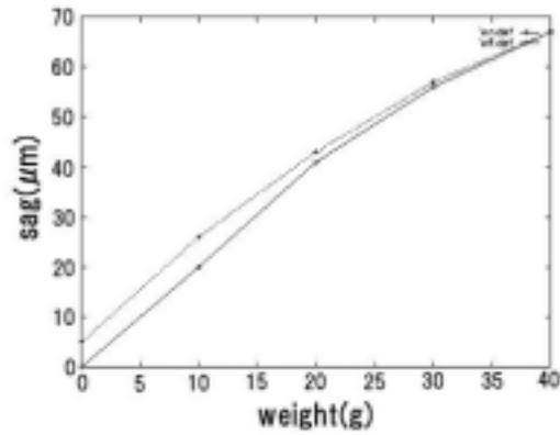
Figure 3.27: The sag of the center of the ladder when we set the weight on the center of the ladder
