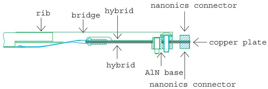
Figure 3.3: Side view of the ladder around hybrid
