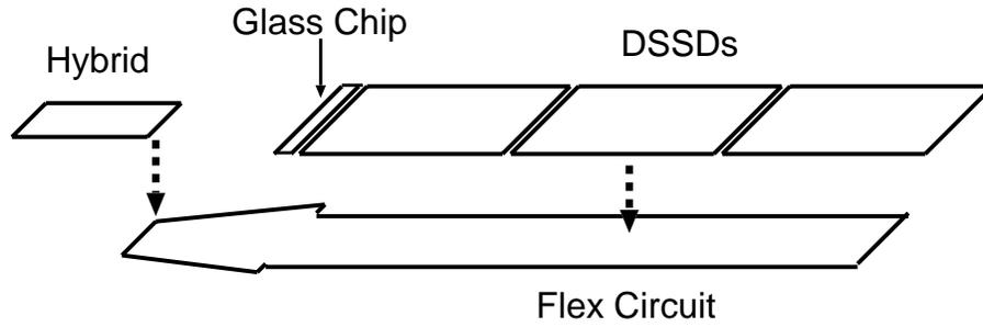
Figure 3.9: Conceptual diagram to glue z-flex to Hybrid and DSSDs
