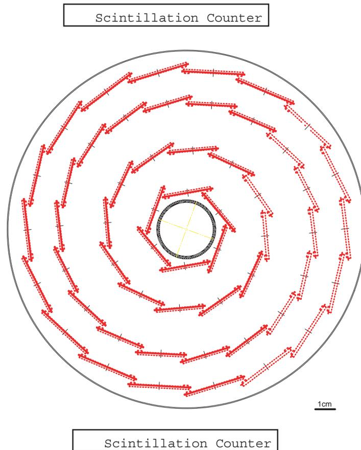
Figure 4.4: Configuration of cosmic ray test (solid lines indicate mounted ladders, and broken lines indicate unmounted ladders)
