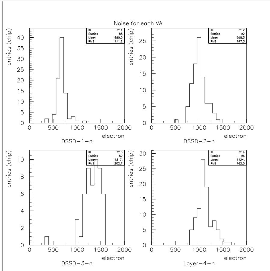
Figure 4.2: Average noise of each VA1TA chip connected to the n-side of DSSD. Results are shown in each half-ladder type: one (top-left), two (top-right), three (bottom-left) DSSD in layer 1-3, and layer-4 (bottom-right).
