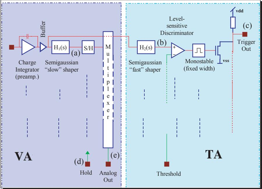
Figure 2.8: VA1TA principle
