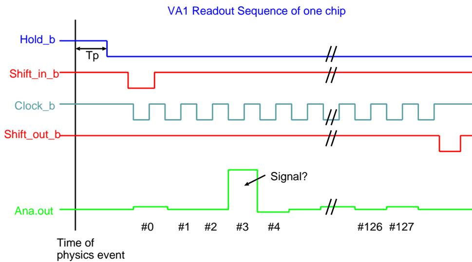
Figure 2.9: Readout sequence of VA1TA
