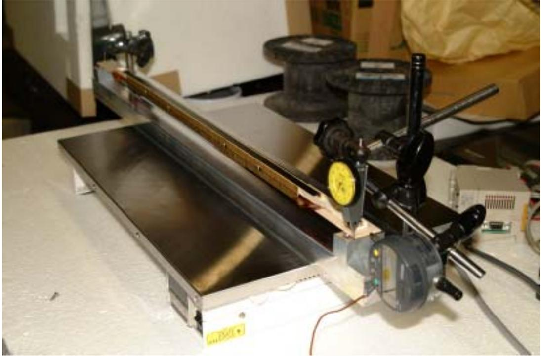
Figure 3.24: Test set up for sliding mechanism
