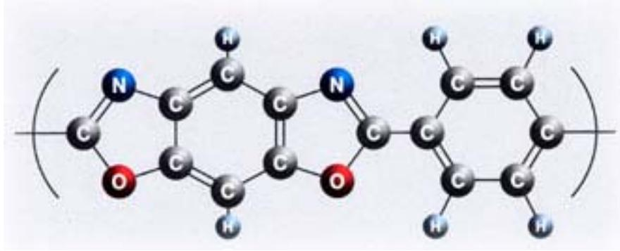
Figure 3.7: Chemical Structure of ZYLON
