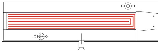
Figure 3.10: Z-flex jig and gluing position
