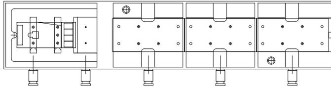
Figure 3.11: Jig to align and fix DSSDs and hybrid pair (DSSD/hybrid jig)
