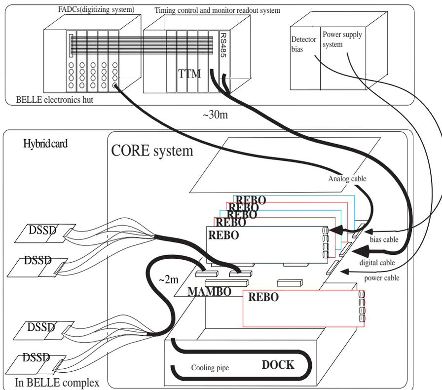
Figure 2.6: Block diagram of the SVD2 readout system
