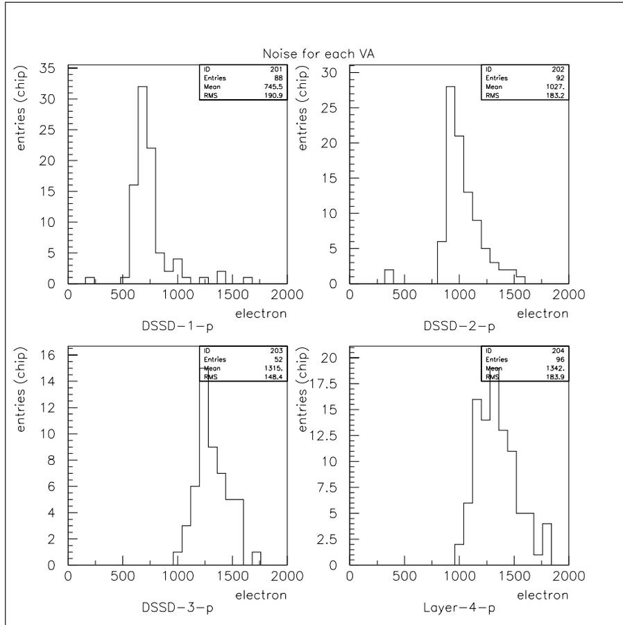
Figure 4.1: Average noise of each VA1TA chip connected to the p-side of DSSD Results are shown in each half-ladder type: one (top-left), two (top-right), three (bottom-left) DSSD in layer 1-3, and layer-4 (bottom-right).
