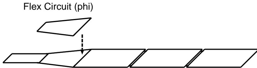
Figure 3.13: Conceptual diagram to glue  $\phi$ -flex
