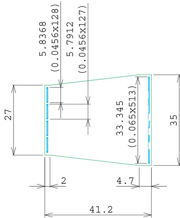
Figure 2.5: Flex circuit (for layer-4  $\phi$ -side)
