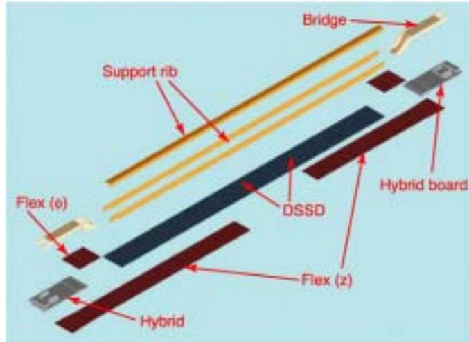
Figure 3.2: Schematics of the components of a ladder
