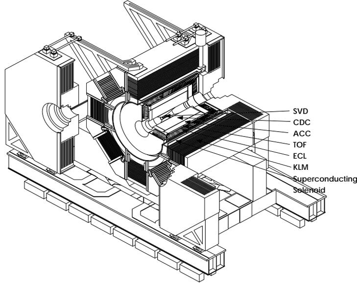
Figure 1.3: Schematic view of the Belle detector
