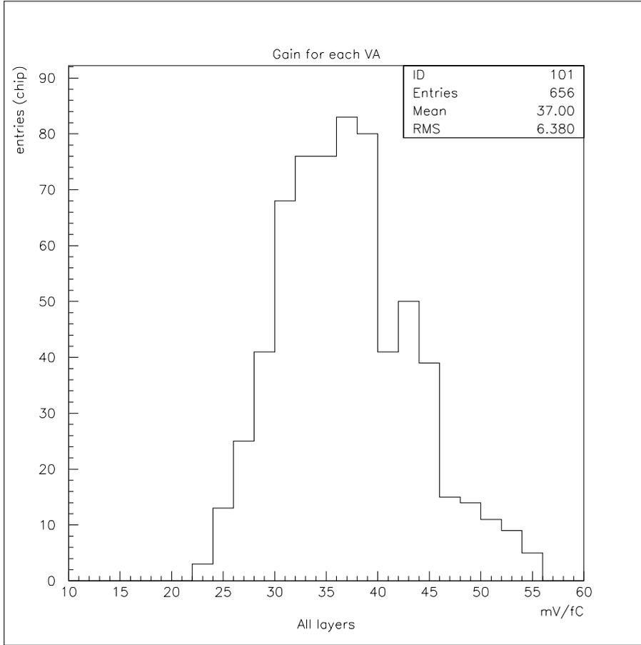
Figure 4.3: Average gain of VA1TA chip
