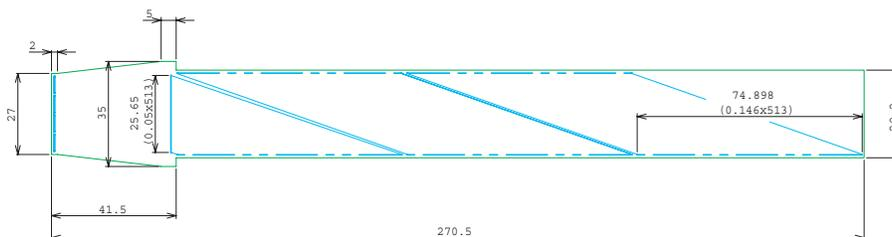
Figure 2.4: Flex circuit (for layer-4  $z$ -side)
