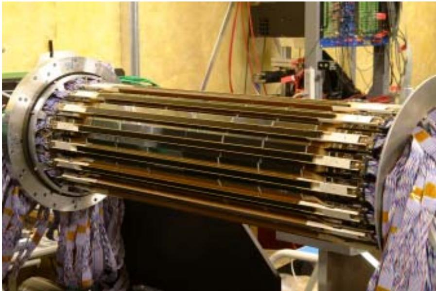
Figure 3.19: SVD2 (ladder mount completed)
