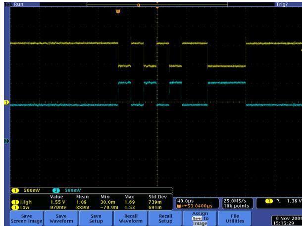
Figure 5.2: UART pattern observed with an oscilloscope. The yellow line is the positive side of LVDS signal, while the blue is the negative side.
