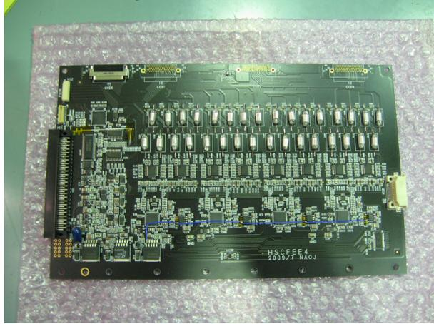
Figure 3.3: FEE board for four CCDs
