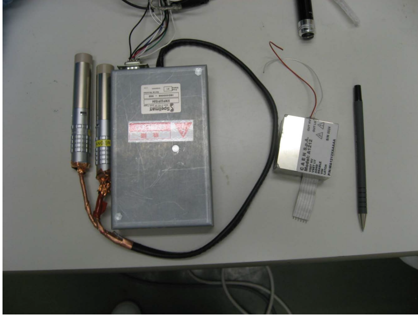
Figure 4.3: Comparison between the HV power supply of the digital HAPD and an ordinary one. The right is the HV system for the digital HAPD.
