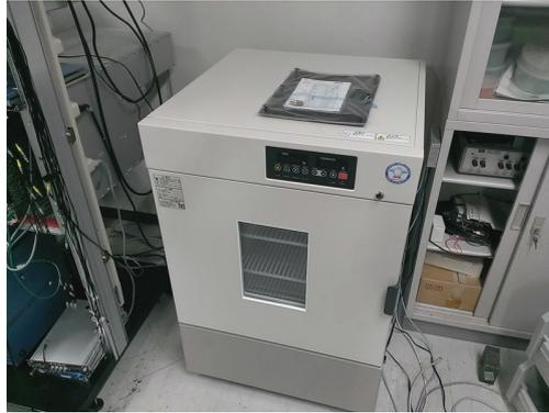
Figure 4.5: Temperature controlled chamber.
