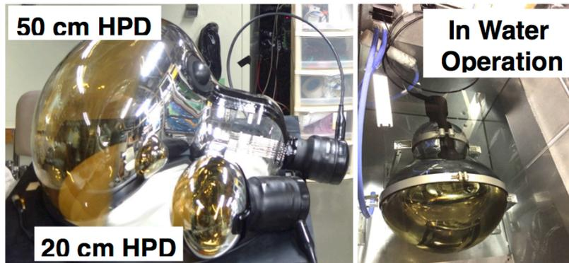
Figure 4.21: The waterproof HPDs and the picture of operation in water.
