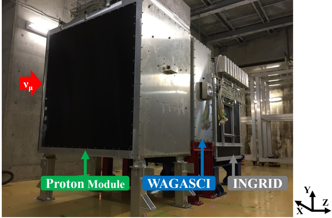
Figure 4.21: Installed detectors at the B2 floor in the J-PARC neutrino monitor building. The coordinate system used in this note is shown: The beam axis corresponds to Z axis.
