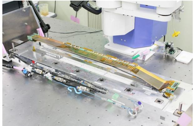
Figure 4.16: Left shows when we attach the Origami parts on the ribs, and right shows after the attachment of the Origami parts.
