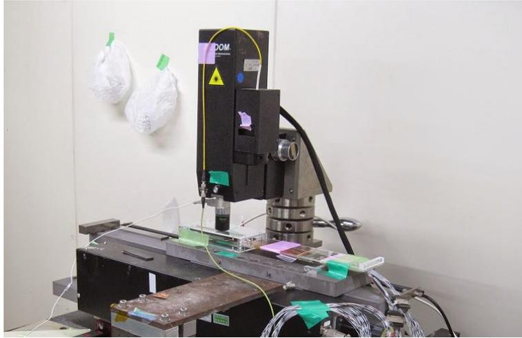
Figure A.9: Laser scan for Single-DSSD module.
