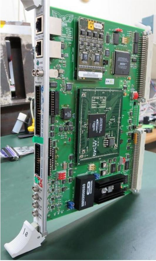
Figure 3.20: The APVDAQ VME board. We use totally three APVDAQ boards; two boards are used to read out p-side, and one board is used to read out n-side signals.
