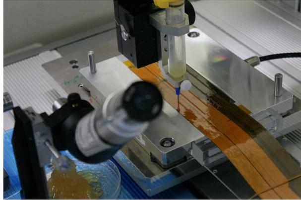
Figure 4.5: Putting glue on the Origami flex
