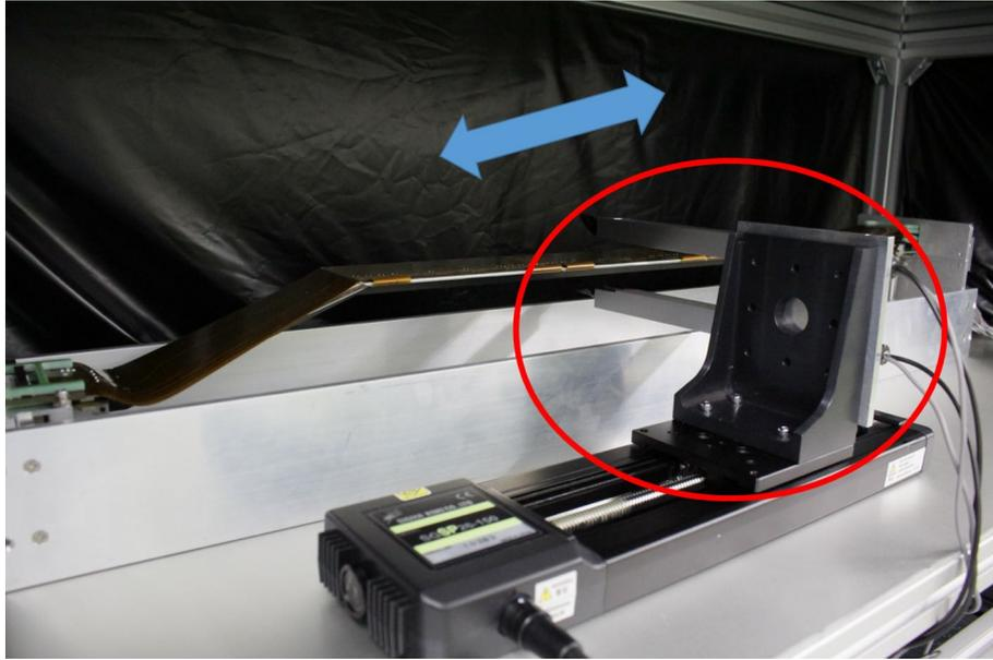
Figure 8.5: Movable stage and prototype SVD ladder (Class-D). This movable stage moves through the DSSD horizontally and allows us to scan all strips in the DSSD.
