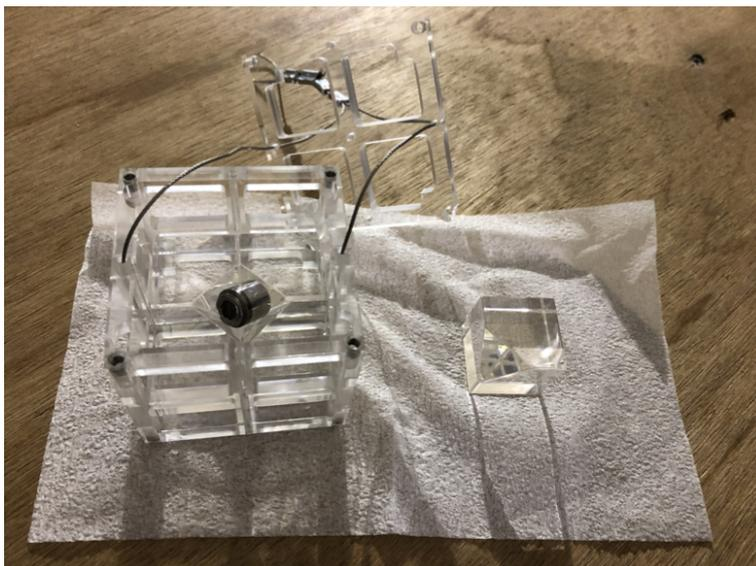
**Figure B.1:** Am/Be neutron source and BGO crystal. The black cylinder in the center on the left is the Am/Be source, and it is assembled by surrounding it with 8 BGO scintillators on the right.
