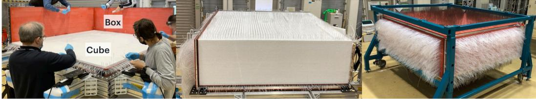
(a) Left: Cube layer stacking, middle: The cube layer stacking finished, right: After closing box
