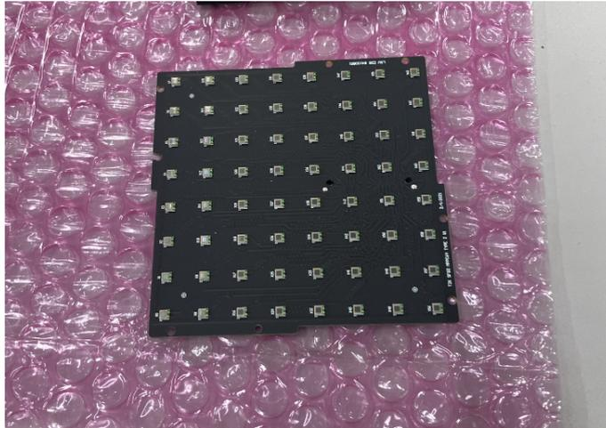
**Figure 3.3.**  $8 \times 8$  MPPCs mounted on a PCB.
